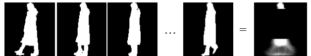
Fig. 6. Modified gait energy image created from a sequence of binary silhouettes (subject 22 of the dataset)
